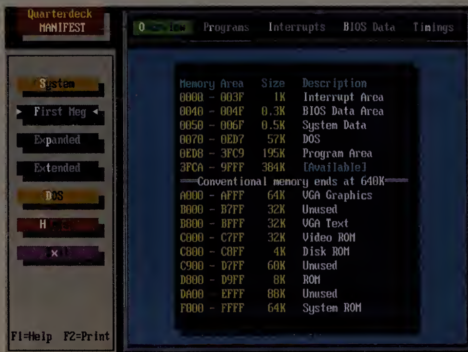
Bundled into Quarterdeck's memory-management offerings, the Manifest utility lets you see precisely what's happening within your computer's memory.
